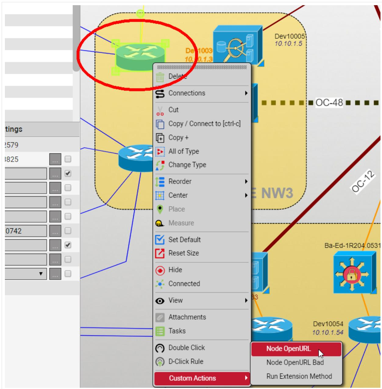
All custom actions are defined in an xml file located in C:\ProgramData\Graphical Networks\netTerrain\vis\CustomActions\CustomUserActions.xml
